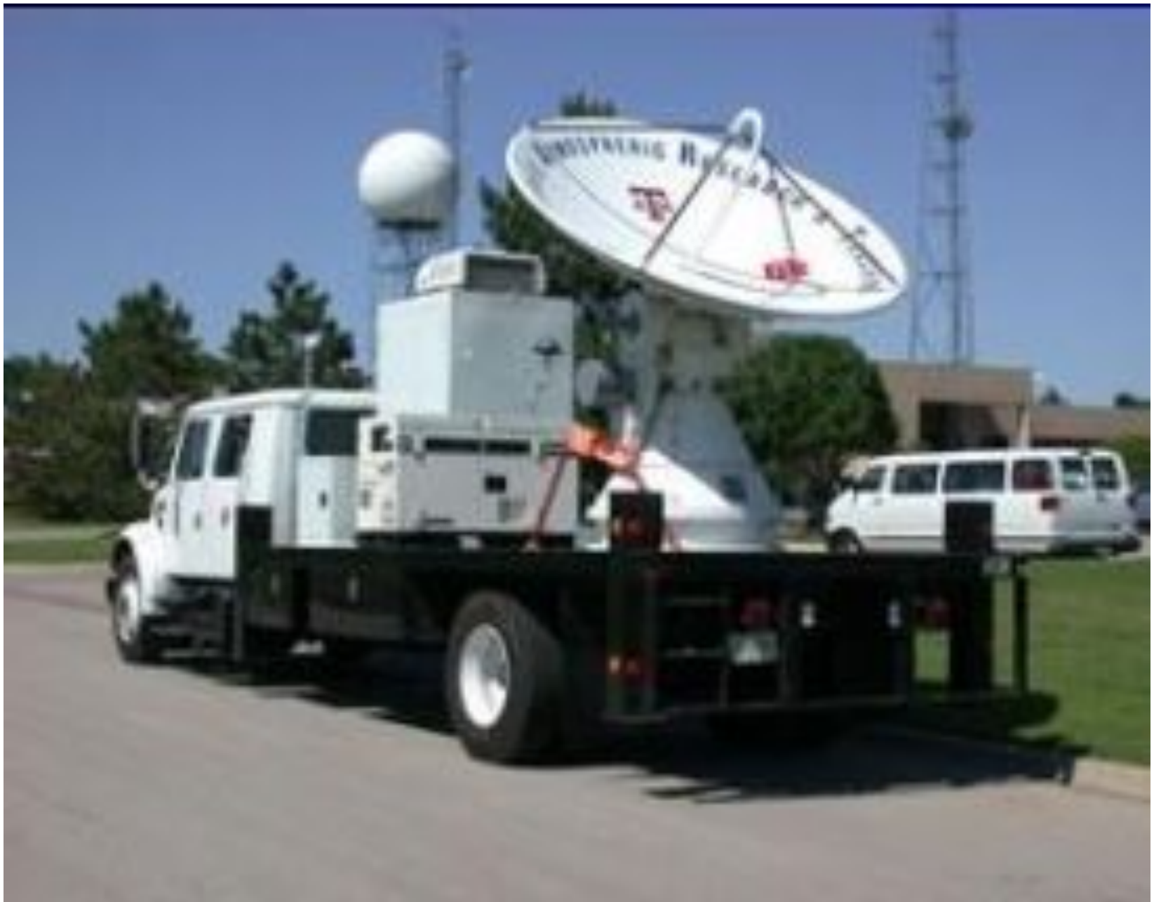
Radar Banda-C ( \lambda = 5 \text{ cm} )
